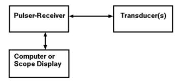
The pulser section of the instrument generates short, large amplitude electric pulses of controlled energy, which are converted into short ultrasonic pulses when applied to an ultrasonic transducer. Most pulser sections have very low impedance outputs to better drive transducers. Control function associated with the pulser circuit include
